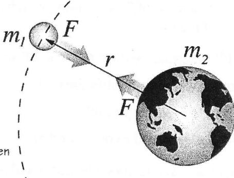
So, when the masses  $m_1$  and  $m_2$  are given in kilograms and the distance  $r$  is given in meters, the force has the unit of newtons. Remember that the distance  $r$  corresponds to the distance between the center of gravity of the two objects.
