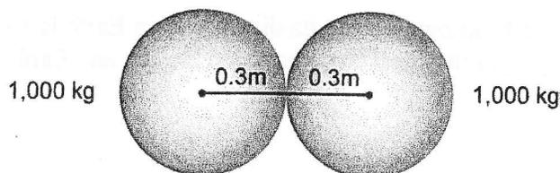
For example, the gravitational force between two spheres that are touching each other, each with a radius of 0.3 meter and a mass of 1,000 kilograms, is given by:
