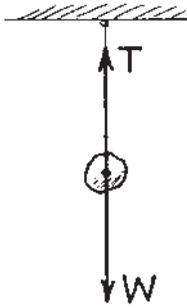
The rock hangs at rest from a single string. Only two forces act on it, the upward tension  $T$  of the string, and the downward pull of gravity  $W$ . The forces are equal in magnitude and opposite in direction.
