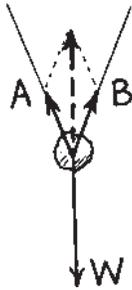
Here the rock is suspended by 2 strings. Tension in each string acts in a direction along the string. We'll show tension of the left string by vector  $A$ , and tension of the right string by vector  $B$ . The resultant of  $A$  and  $B$  is found by the **parallelogram rule**, and is shown by the dashed vector. Note it has the same magnitude as  $W$ , so the net force on the rock is
