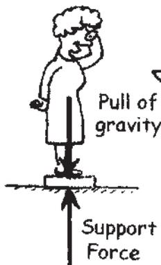
When I step on a weighing scale, two forces act on it: a downward pull of gravity, and an upward support force. These equal and opposite forces effectively compress a spring inside the scale that is calibrated to show weight. When in equilibrium, my weight =  $mg$ .
